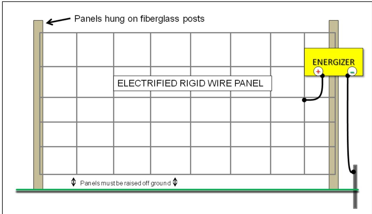
*Figure 6. Electrified rigid wire panel. The panel is raised off the ground and insulated by hanging it from fiberglass posts. The wire panel is electrified by connecting it directly to the positive terminal on the energizer. The ground rod is connected to the negative terminal of the energizer.*
